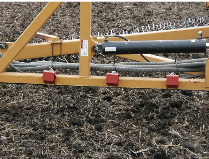
Rotary Harrow Seeding - seed delivery ports
