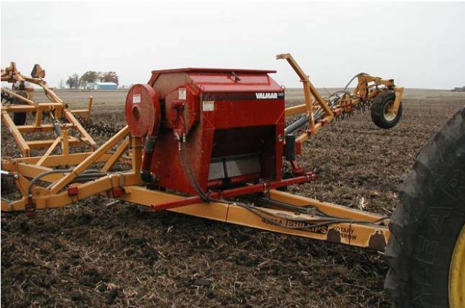
Rotary Harrow Seeding - mounted air delivery seeder in light residue crops
