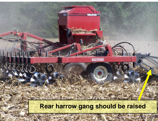
Coultter Harrow (vertical tillage tool) Seeding - air delivery seeder on a coultter harrow in heavy residue crops
